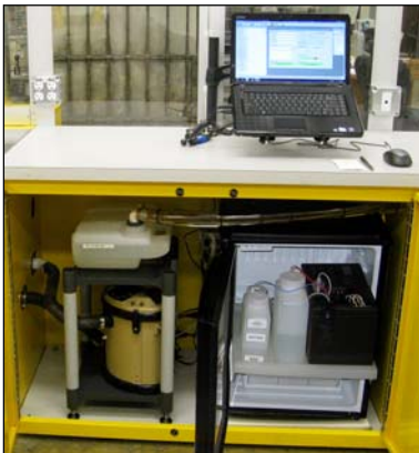
ASAP II System showing SASS 2300 air sampler with RAPTOR bioassay module.
