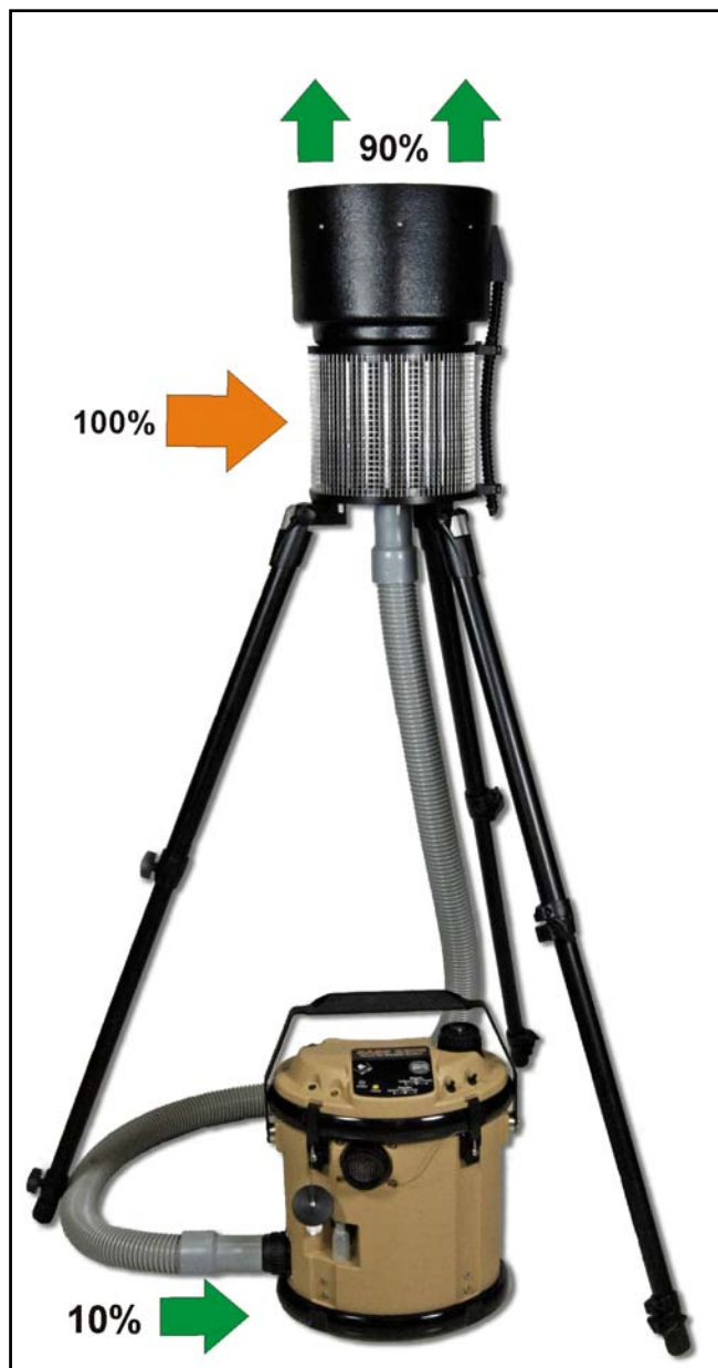
Figure 3: Airflow patterns for the SASS 4000 Concentrator.
