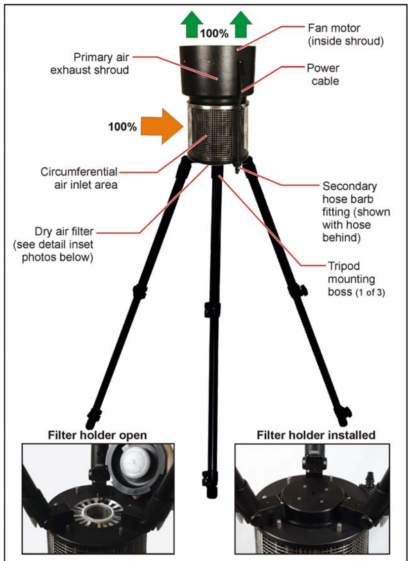
Figure 3: Airflow patterns for the SASS 4100 two-stage aerosol collector.
