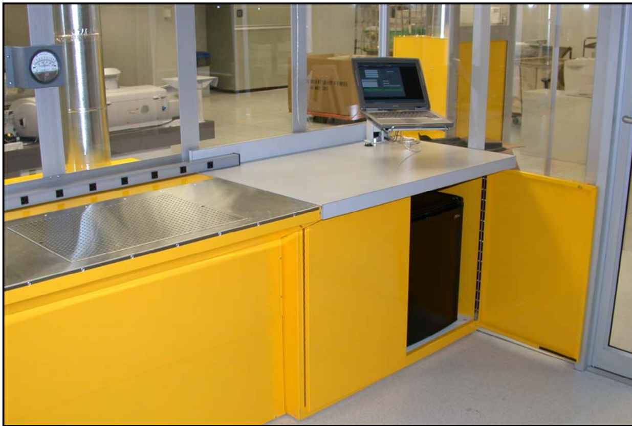
Downdraft table with open cabinet door where ASAP II system is located. The laptop computer on which ASAP II control software is installed is also shown.
