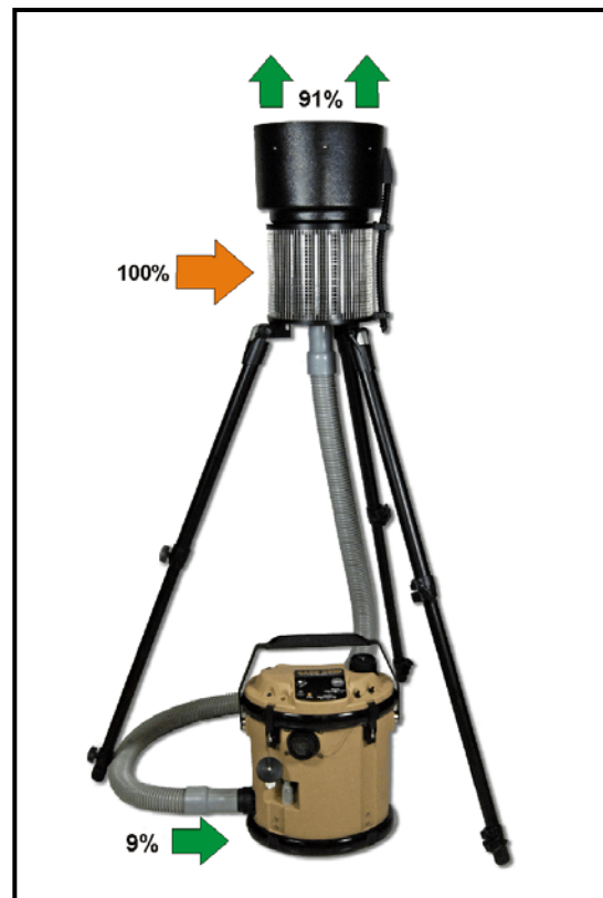
Figure 1: SASS 4000 Plus Concentrated Wet Air Sampling System showing air flow patterns.
