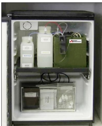
ASAP II environmental cabinet with RAPTOR, buffer and waste bottles, and supplies storage.
