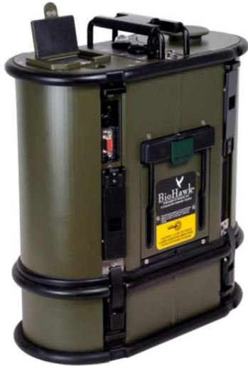
BioHawk 8-channel collection and bioidentification system
