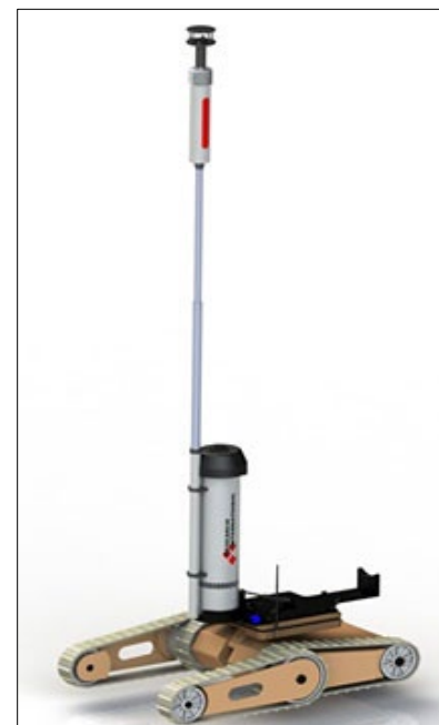
Robotic mounting method for Remote Sensor Node, shown in active/field use position.
