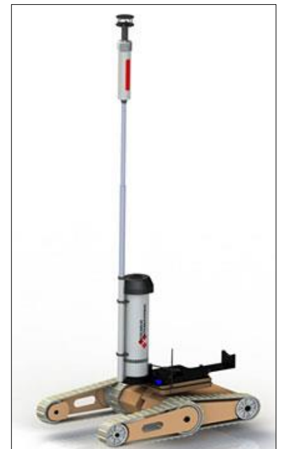
Robotic mounting method for Remote Sensor Node, shown in active/field use position.
