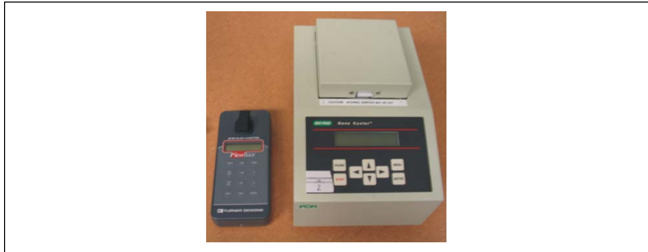
Figure 3: An Example of a Portable Thermal Cycler and a Handheld Fluorescence Reader Provided
