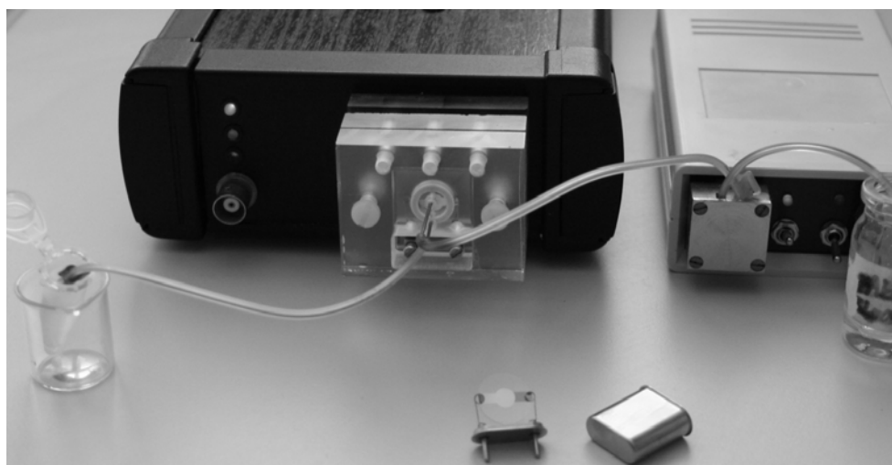
Fig. 3. The compact piezoelectric immunosensor (left) with integrated flow-through cell. The flow of solutions is realized using the miniperistaltic pump (right). The exchangeable piezoelectric quartz crystal is shown in front.
