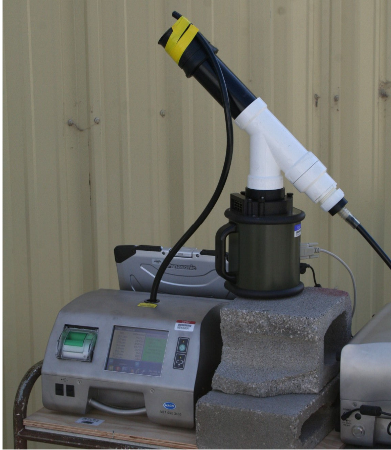
Figure 1- Sampler and particle counter set-up (ambient test).
