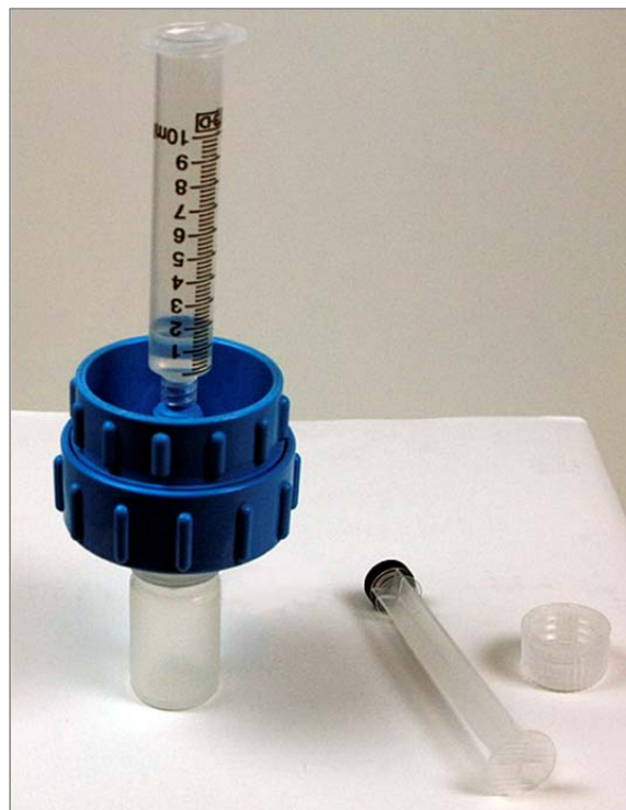
Figure 2: Assembled filter holder with an attached syringe barrel containing the extraction fluid.
