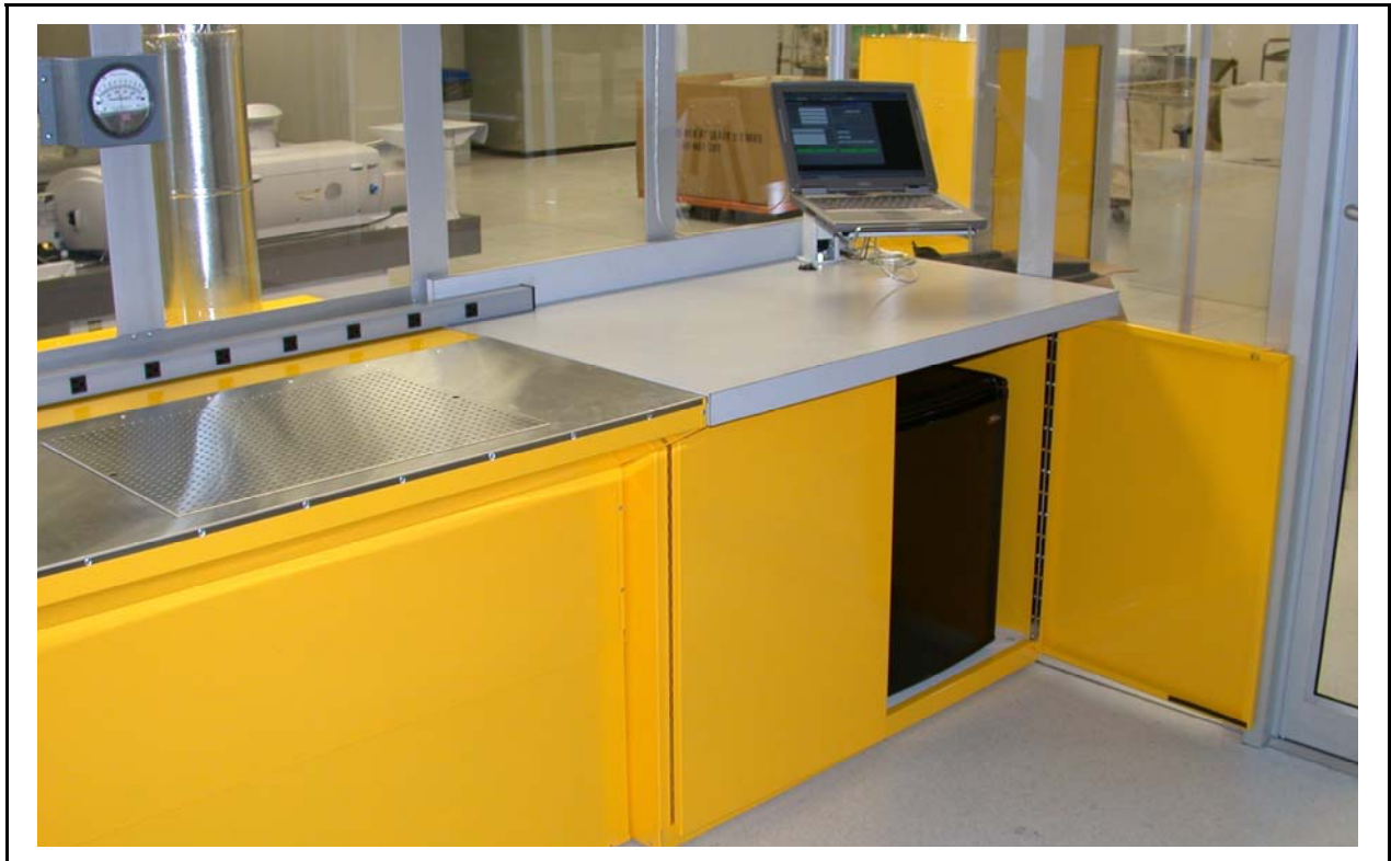
Downdraft table with open cabinet door where ASAP II system is located. The laptop computer on which ASAP II control software is installed is also shown.
