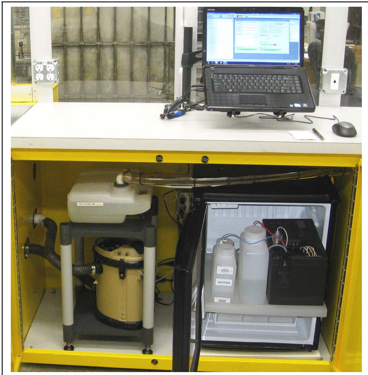
Cabinet space below downdraft table, which houses SASS air sampler on the left and environmental chamber where RAPTOR or BioHawk module is located, on the right.
